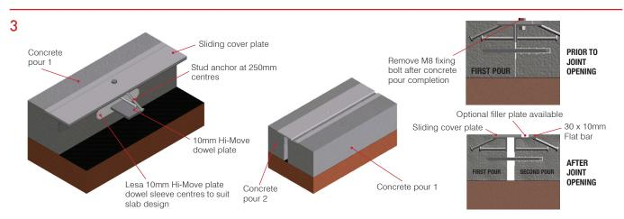
NOTE: Top mount bolt is optional and made to order. Steel sizes in above drawings are for Type G45.
