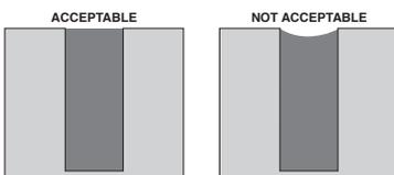
To be effective as an edge-protector, **RS 88**'s final profile should be flush with the floor surface. This is achieved by razoring off the overfill crown after the **RS 88** has fully cured into a solid. If **RS 88** is gummy or liquid when shaving, allow additional cure time.
