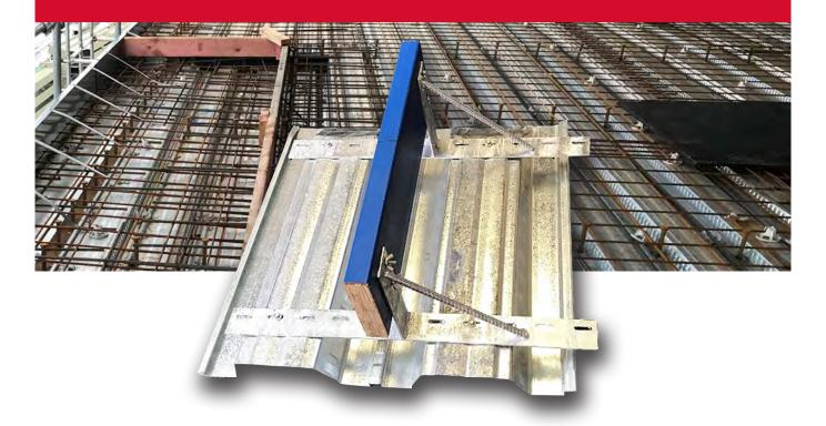
The **LESA Composite Floor Bracket System** was developed to speed up construction when forming set-downs on Comflor and Tray-dec Suspended Composite Flooring Systems. The **LESA Composite Floor Bracket System** is a stay in place galvanised bracket that enables the contractor to achieve a monolithic pour (pouring the set-down area of the slab at the same time as the main slab even though the two slabs are at different elevations).
