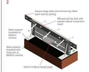
3 Square edge steel joint armouring offset each end for joining M8 special hex bolt with washer-lateral movement insert Stud anchor at 250mm centres Lesa 10mm Hi-Move dowel plate Steel support brackets at 600mm centres Lesa 10mm Hi-Move plate dowel sleeve centres to suit slab design
